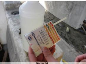
Discharge from site shall not endanger public health or causing harm to the sewerage or drainage system. Water sample was collected and tested for compliance with the safety standard.
