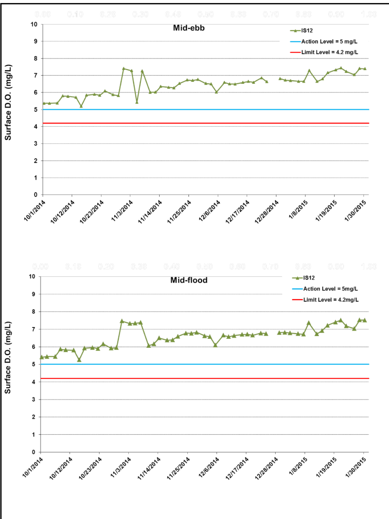
Figure I3 Impact Monitoring - Mean Level of Dissolved Oxygen (mg/L) in surface waters between 1 October 2014 and 31 January 2015 at IS12. The weather conditions during the monitoring period varied mostly from sunny to cloudy. Major marine construction activities included: Construction of Temporary Seawalls (10/1/2014 - 11/20/2014); Sheet Piling (10/1/2014 - 11/20/2014); Filling (10/1/2014 - 11/20/2014). WQM on 26 December 2014 was postponed to 29 December 2014. Ref: 0212330_Impact-WQM_January2015_graphs_Rev a.xls
