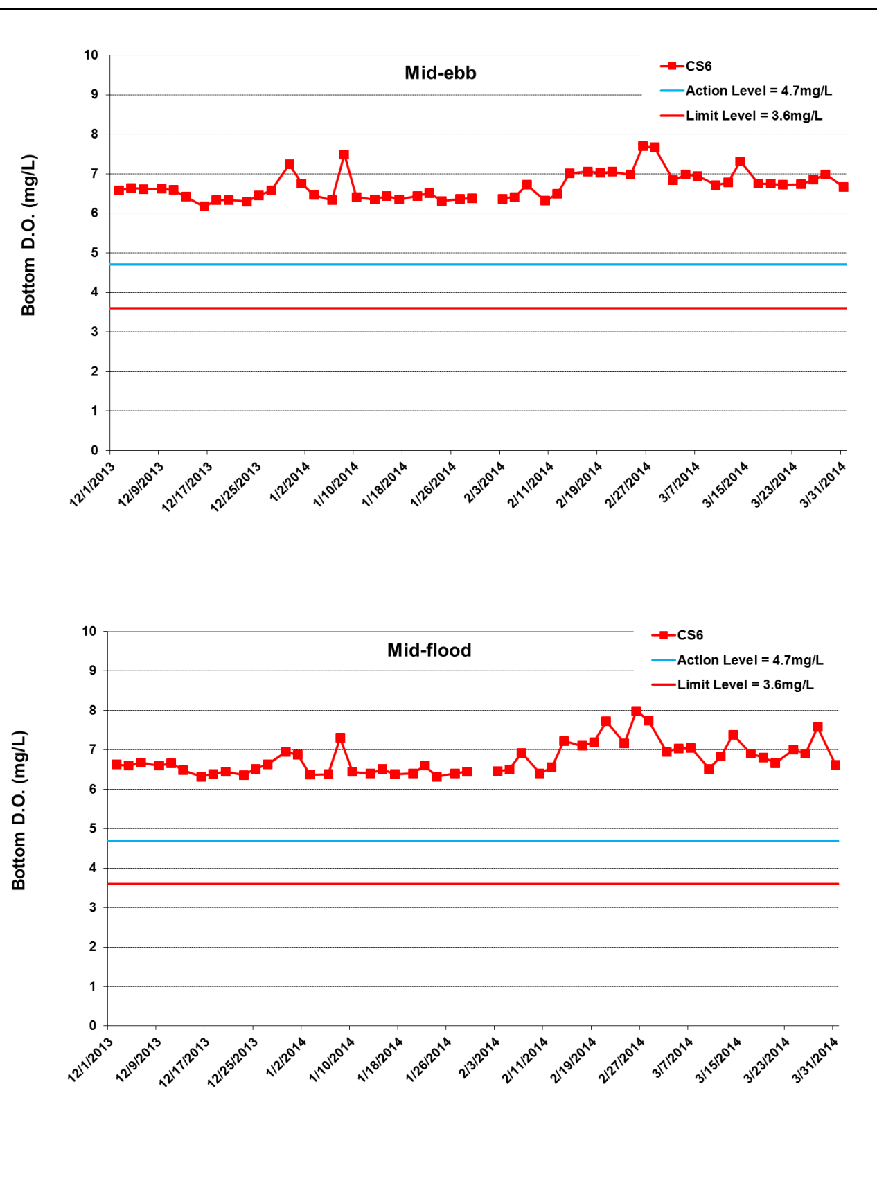
Figure I18 Impact Monitoring - Mean Level of Dissolved Oxygen (mg/L) in bottom water between 1 December 2013 and 31 March 2014 at CS6. Note no dredging/ filling works was undertaken on 31 January 2014.
